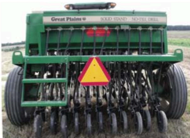
The use of a no-till drill can help with seed placement and soil-to-seed contact to improve total germination and seedling survival on tough, dryland soils.
