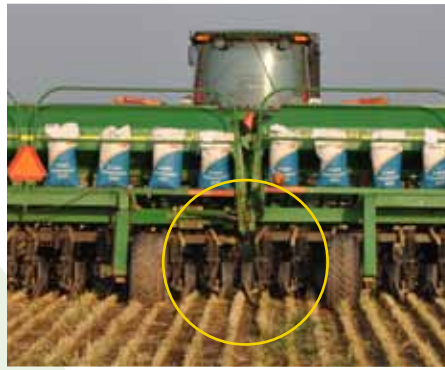
Press wheels, especially for no-till seeding helps produce full, uniform stands, especially when soil moisture may be limited.
